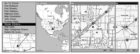
Map Menu with Resize Window command selected (left). Pressing  $\rightarrow$  moves the centerline and enlarges the left window (right).
